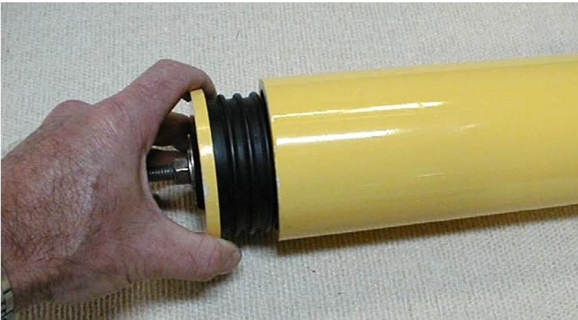
**Figure 1 Removing hull seal plug**
