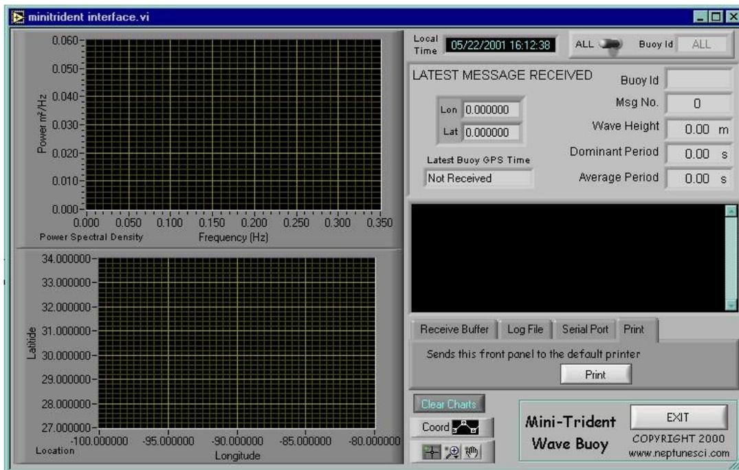
2. You can select display and graph results from "ALL" the buoys active or just display a specific buoy by flipping the Buoy Selection switch. Note: All messages received from all active Mini Sentry buoys are stored to the log file regardless of this setting. This switch only affects which buoys are displayed.
