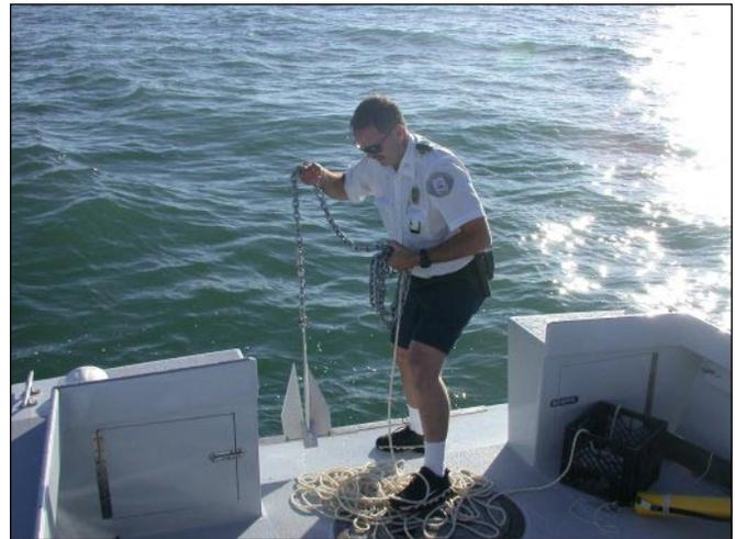
**Figure 31** Maintain tension on the mooring line during recovery (l) until the anchor is aboard (r).
