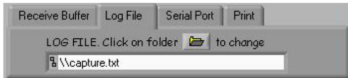
**Serial Port:** This control is used to select a serial port to use to communicate to the radio transceiver. You will not need to modify this control unless you changed ports since you started this session.
