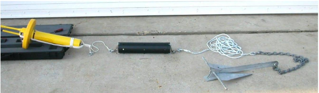
**Figure 22 Buoy attached to mooring, ready for deployment**
