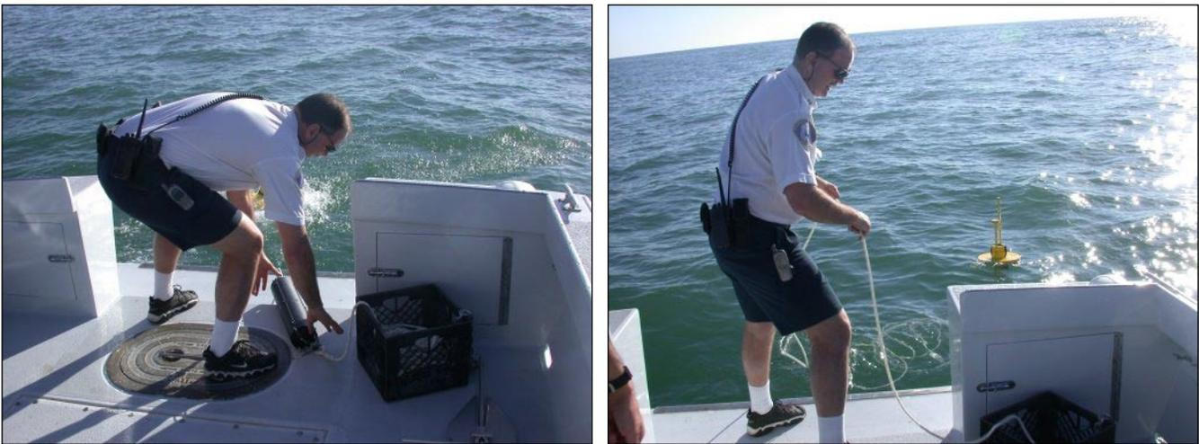
**Figure 29** During deployment, pay out the buoy and sea anchor first, then the mooring
