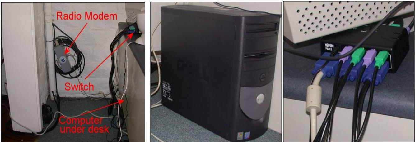
Figure 27 Base station modem (l), computer (c), and switch (r).
