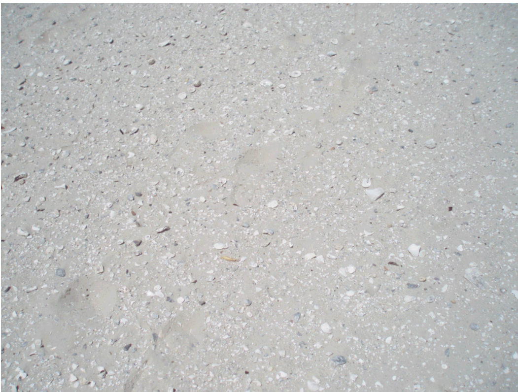
Close-up of self-armor by shell fragments. Note how easily footprints disturb the armor layer.
