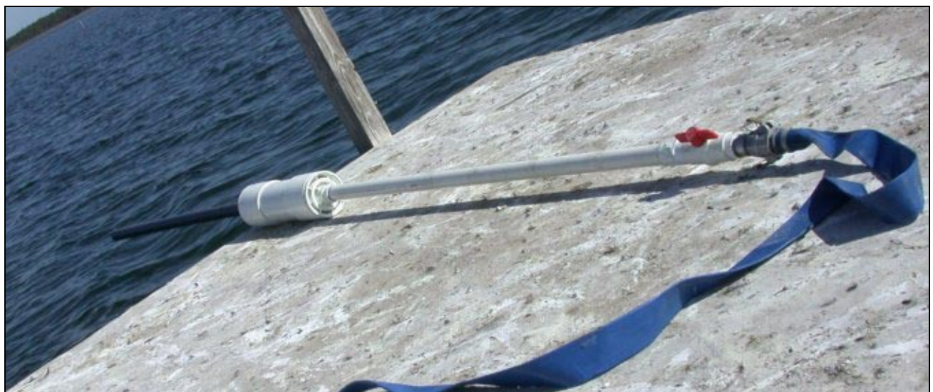
Figure 5 - Gage Mount with Fixed Pile and Deployment Pipe Attached
